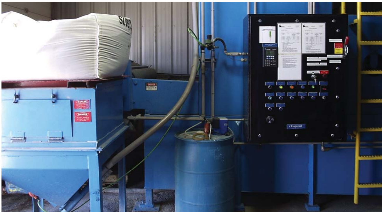
Prokleen Washing Services, diversion and reuse of final rinses reduces clay consumption and solid waste generation in the wastewater treatment plant by 118 tonnes/yr. An alternate dewatering process can reduce solid waste by an additional 190 tonnes/yr.
