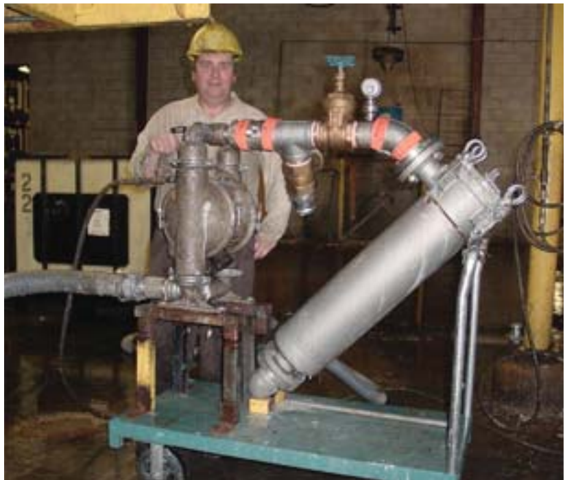
Halltech Inc., closed-system product filtration that reduces product loss and sewer use bylaw pollutants, resulting in significant cost savings.
